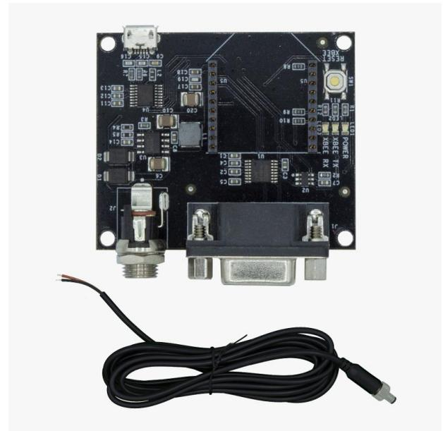
RS232 Carrier Board for XBee Plugins SKU is: AS-ADP-12VRS232-TO-XBEE-01
