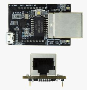
Ethernet NTRIP Master SKU is: AS-XBEE-ETH-100-RJ45-00
