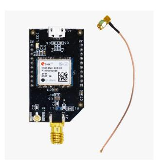
Japan CLAS Corrections L6 Receiver NEO-D9C SKU is: AS-XBEE-LBAND-NEOD9C-SMA-00
