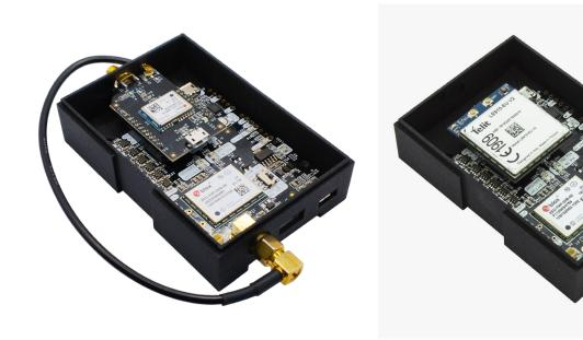
RTK-SSR Receiver with PointPerfect (Internet or L-Band) includes free basic technical support. Contact info@ardusimple.com for more information.
