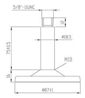
Magnetic Stand for Survey GNSS Antenna includes free basic technical support. Contact info@ardusimple.com for more information.
